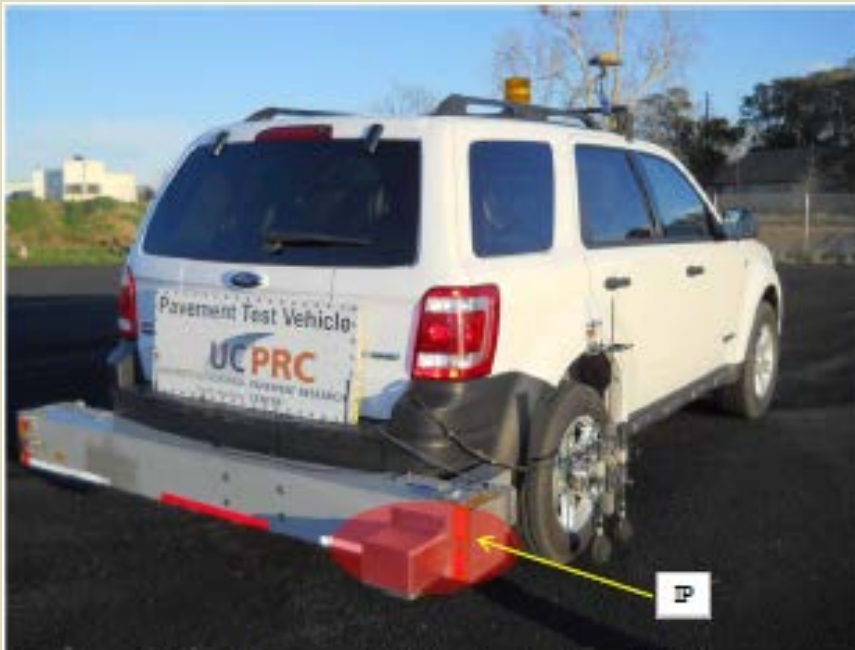
Figure 4.7: Instrumented vehicle with an inertial profiler (IP).
